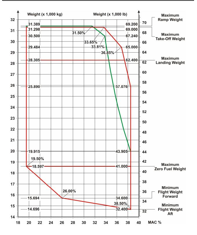
The red line shows the in-flight limits. The green line shows the on-ground limits.
