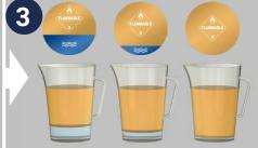
Agitate sample using a swirling motion and leave to **settle for 12-15 mins**. Once settled, is there any free water?
