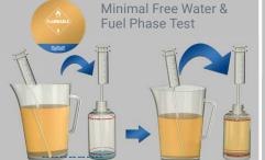
If there is visible free water but not enough to reach the '**Water line**' when syringed into the FUELSTAT® test bottle, continue syringing fuel from near the bottom of the sample up to the top line marked '**Fuel line**'
