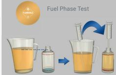
If there is no visible free water in the sample, syringe fuel from near the bottom of the sample into the FUELSTAT® test bottle up to the top line marked '**Fuel line**'
