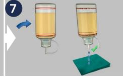
Fully invert the bottle and allow 4 drops to spill onto a tissue to clear the dropper nozzle of any trapped fuel deposits, **DO NOT TURN THE BOTTLE UPRIGHT**
