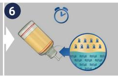
Invert test bottle 45° and allow the blue fluid to settle out in the shoulder of the bottle. NOTE: for a free water phase only test the blue fluid will not separate out
