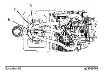
**3.** Remove bolts (6), plate (7), tank manifold (8), and gasket (not shown).
