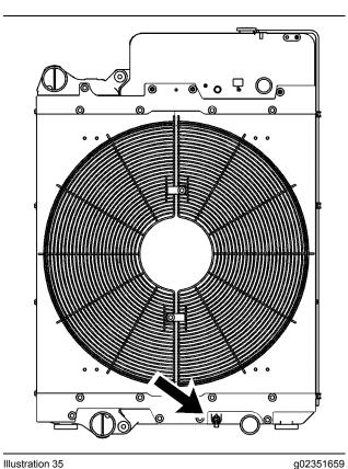
The cooling system drain valve is towards the bottom of the radiator.
