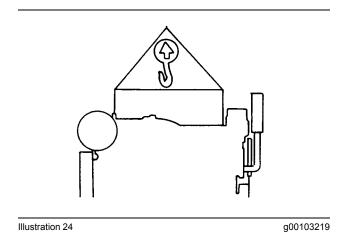
NOTICE Never bend the eyebolts and the brackets. Only load the eyebolts and the brackets under tension. Remember that the capacity of an eyebolt is less as the angle between the supporting members and the object becomes less than 90 degrees.
