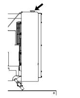
Illustration 37 Cooling system filler cap
