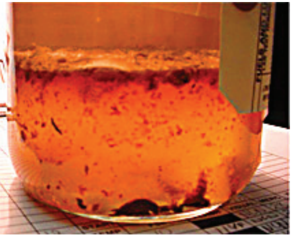
Fuel contaminated with fungal growth. This infestation can occur in aircraft fuel tanks causing clogged filters and corrosion.
