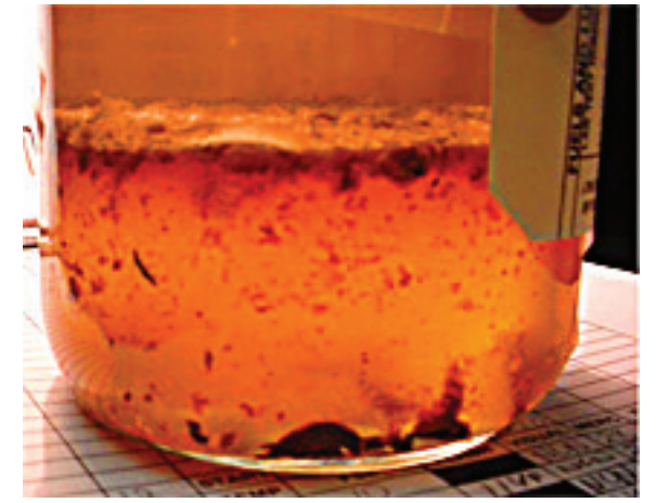
Fuel contaminated with fungal growth. This infestation can occur in aircraft fuel tanks causing clogged filters and corrosion.
